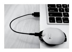
1. Charging is performed with the included USB cable. There is notch in the unit to ensure the connection is in the correct orientation.
